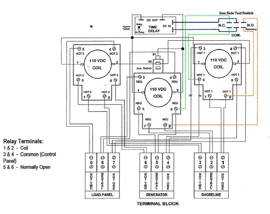
The 100 is intended for use as an electrical transfer switch to automatically switch multiple sources from one to another, such as switching from Shoreline to Generator power.
